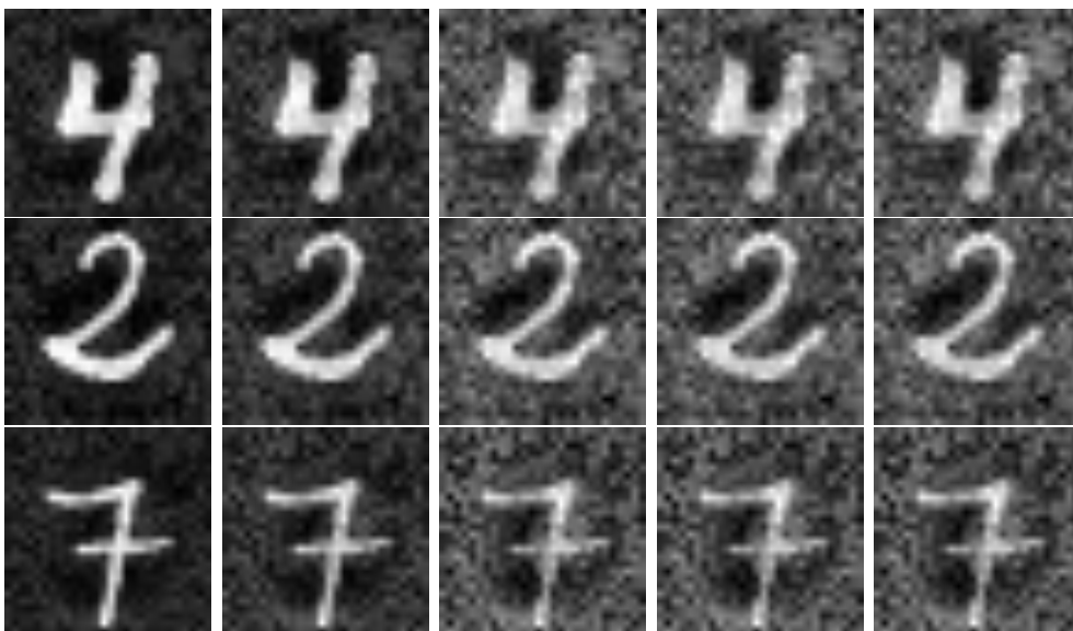
Figure 1.9: Example 6.4.5: We illustrate the evolution of three individual MNIST samples \mathbf{x}_i(t) \in \mathbb{R}^{784} at times t \in \{0, 2, 8, 15, 19\} – each trajectory stabilizes to some steady configuration after time t \geq 8 . Curiously enough, the neural ODE tends to compress the input digit samples ahead of classifying via the softmax applied to the output features P\mathbf{x}_i(t) \in \mathbb{R}^{10} . See Example 6.4.5 for modeling considerations.
