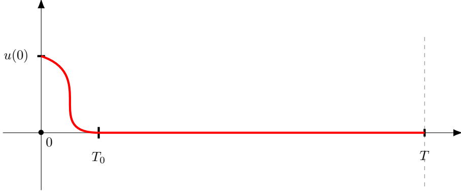
Figure 5.3: Proof of Lemma 5.5.1. The first two terms appearing in (5.5.1) also appear in the functional J_T(u_T) . We thus construct an admissible quasi-turnpike control u^{\text{aux}} (red), for which the corresponding state y^{\text{aux}} (blue) coincides with \bar{y} over (T_0, T) . In this way, as J_T(u_T) \leq J_T(u^{\text{aux}}) , and J_T(u^{\text{aux}}) is independent of T , we can conclude. The estimate of the third term then follows from Lemma 5.4.1.
